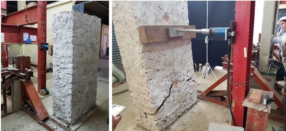
Out of plane pushover test of unreinforced stone in mud wall at IOE lab, Pulchowk
