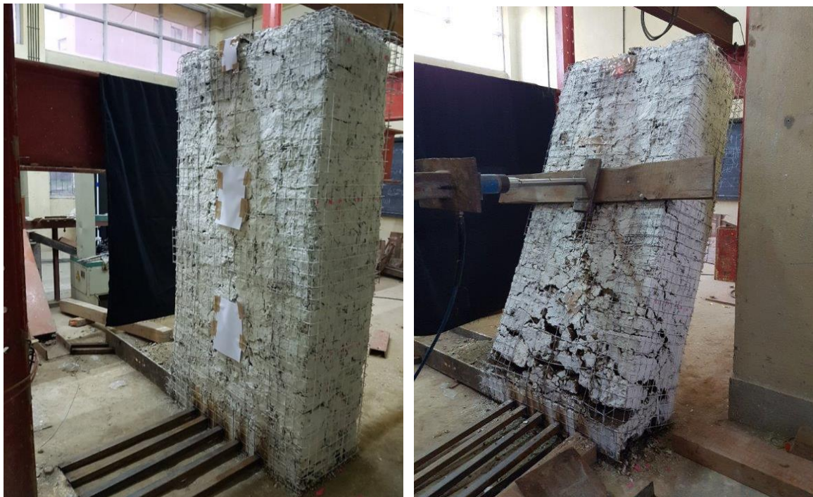
Out of Plane Pushover Test of stone in mud wall retrofitted using wire mesh at IOE lab, Pulchowk
