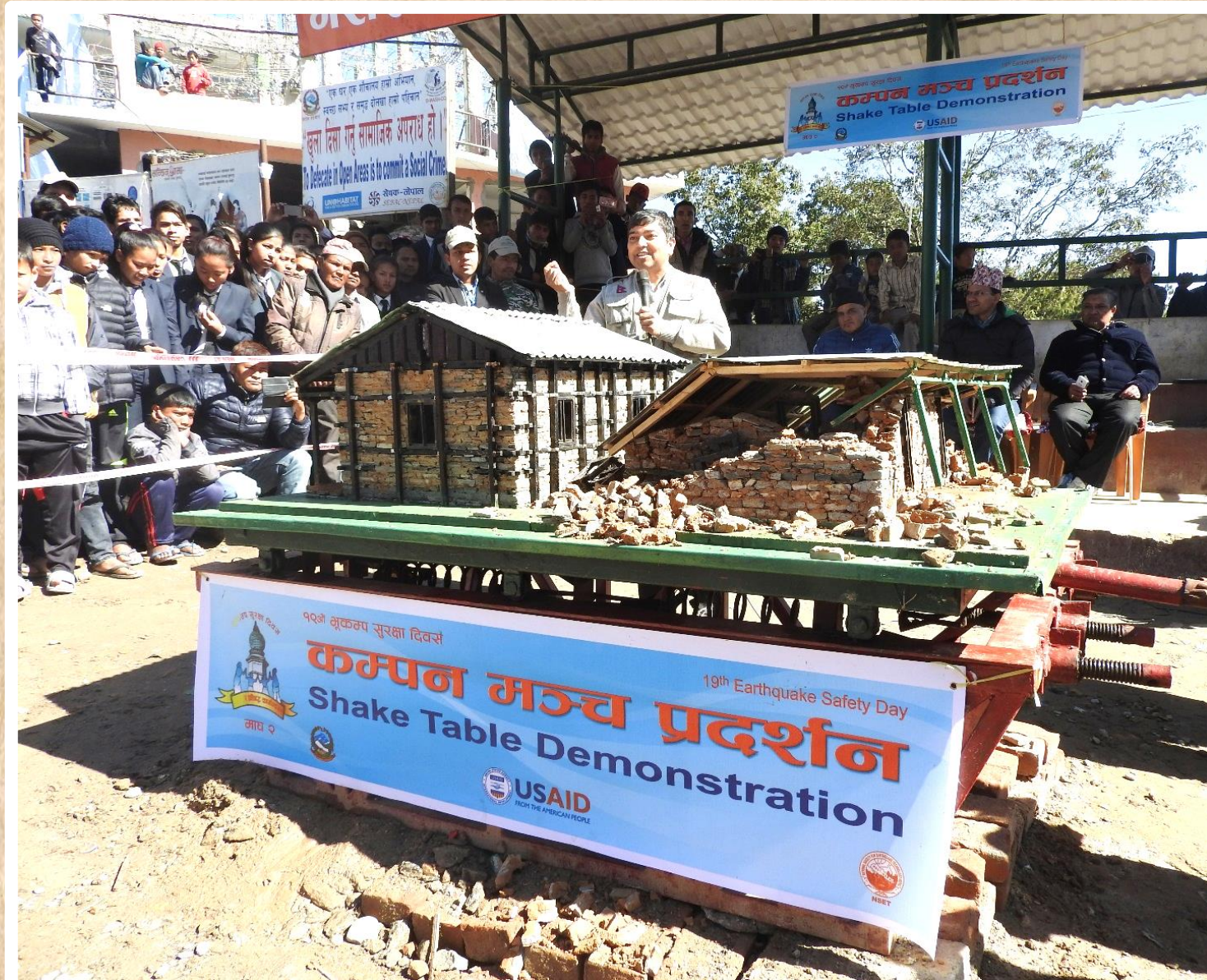
Photo caption: Seeing is Believing ! Awareness through Shake Table Demonstration. Baliyo Ghar Program conducted Shake Table Demonstration in the program areas to convince beneficiaries on how the earthquake safe building behaves during ground shakings. Such demonstrations were conducted occasionally, like in the Earthquake Safety Day and in commemoration of Gorkha Eathquake.
