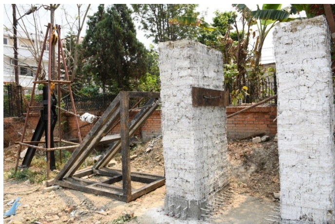
Wall Pull down test of Retrofitted stone in mud masonry walls
