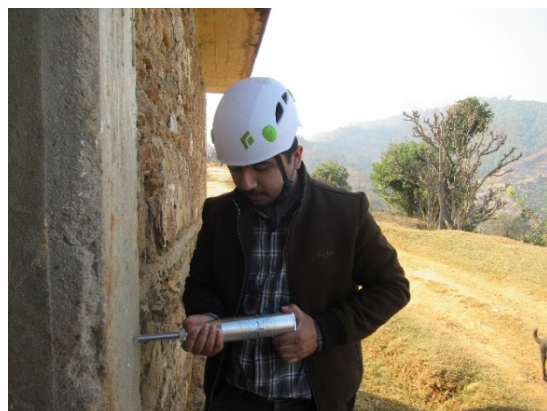
Bar Scanner test to determine the number of reinforcements
