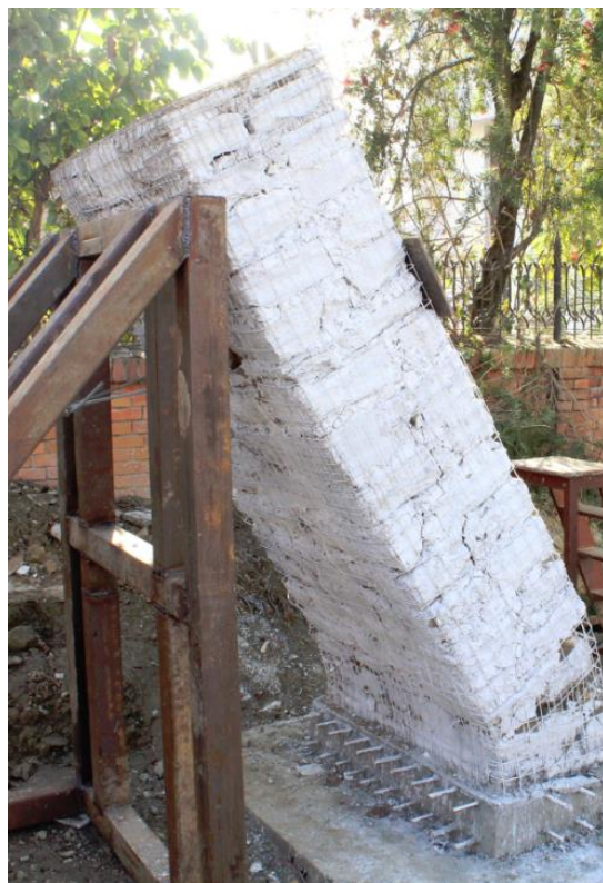
Out of plane pulldown test of stone in mud wall retrofitted using welded wire mesh
