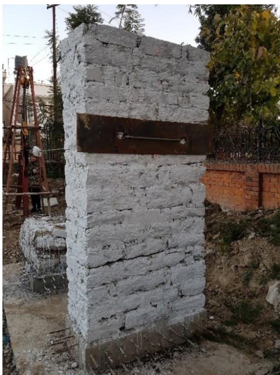
Out of plane pulldown test of non retrofitted stone in mud wall
