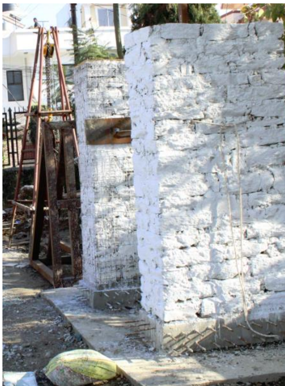
Out of plane pulldown test of stone in mud wall retrofitted using welded wire mesh
