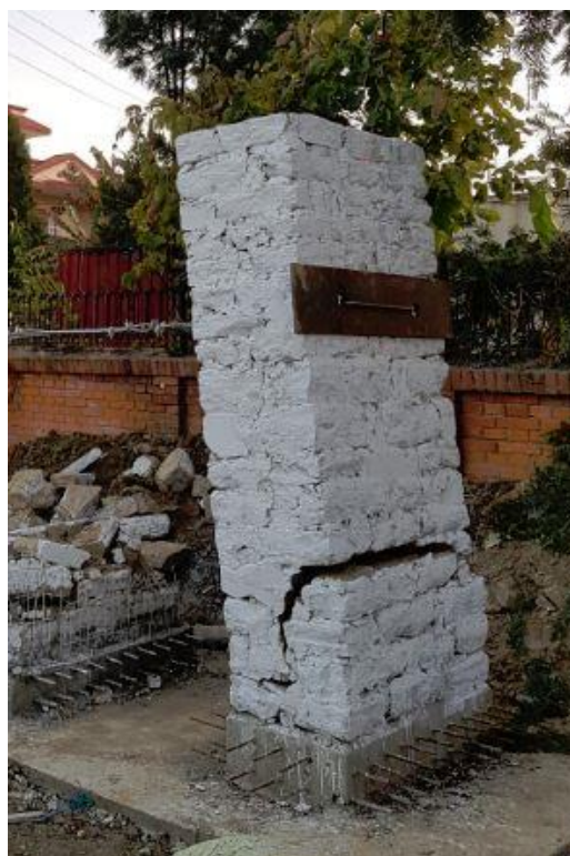
Out of plane pulldown test of non retrofitted stone in mud wall
