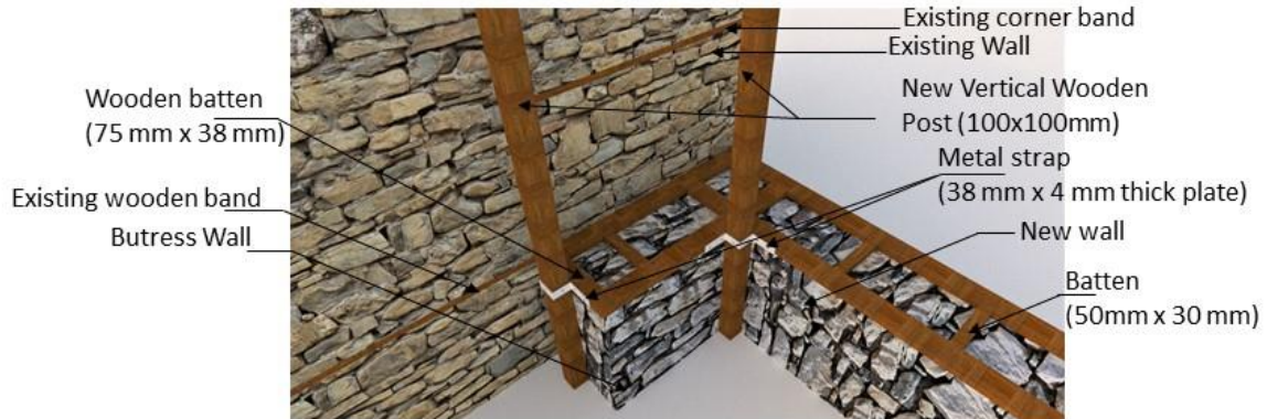
Figure 21. Provision of buttress to stiffen the new wall where cement and reinforcement are not available in case of Stone masonry
