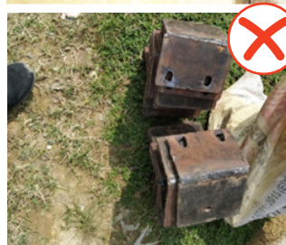
Poor welding connection at site
