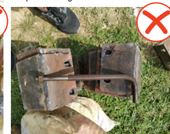
Poor welding connection at site
