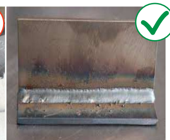
Proper through welding
