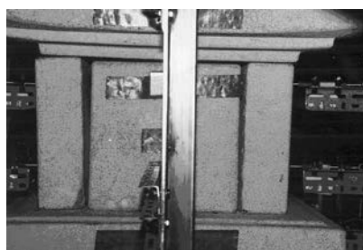
(a) Failure mode I; the initiation of instability at the first storey pagoda body due to sliding
