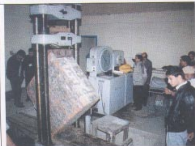
Testing of a 1.2 \times 1.2 \times 0.46 m non-reinforced-masonry-block prototype in Tribhuvan University Laboratory to obtain the diagonal tensional strength (shear strength) in masonry assemblies according to ASTM.
