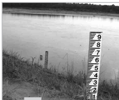
Figure 4.3: Water level-gauge installed at the river bank
