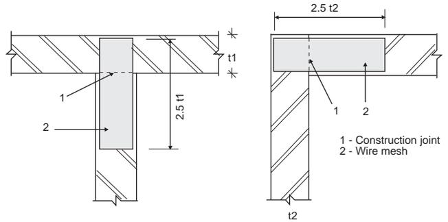
Fig. 33 : Joint strengthening by wire fabric
