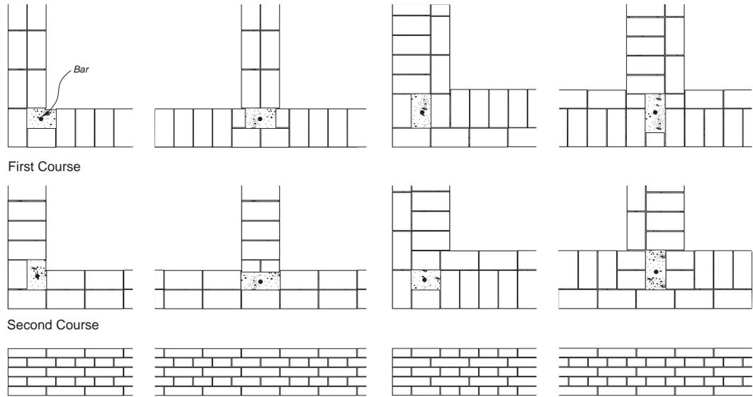
Fig. 36 : Vertical reinforcement in brick wall
