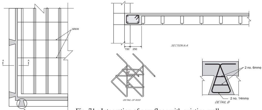
Fig. 71 : Integration of new floor with existing wall
