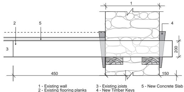
Fig. 63 : Anchorage of timber joists with wall using wedges
