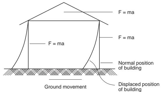
Fig. 10: Ground motion and Inertia force
