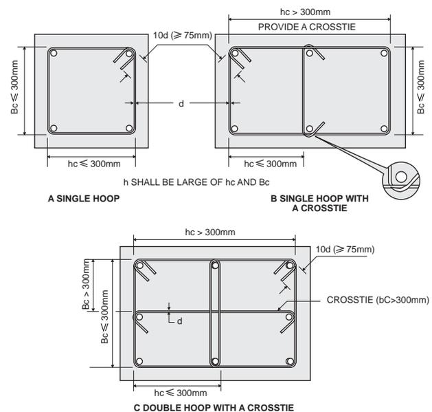
Fig. 57 : Transverse reinforcement in column
