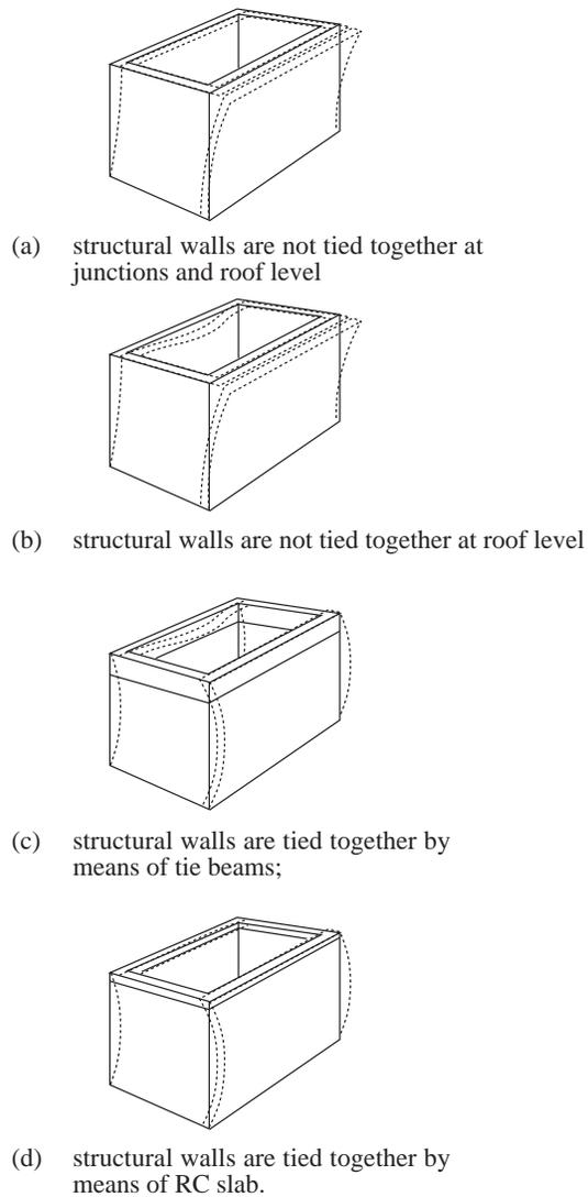
Fig. 12: Vibration of masonry building during earthquake ground motion
