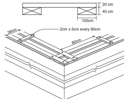
Fig. 48 : Detail of timber band
