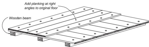
Fig. 64 : Floor stiffening using two layers of planks
