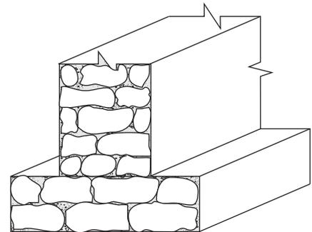
Fig. 26 : Plum concrete strip footing
