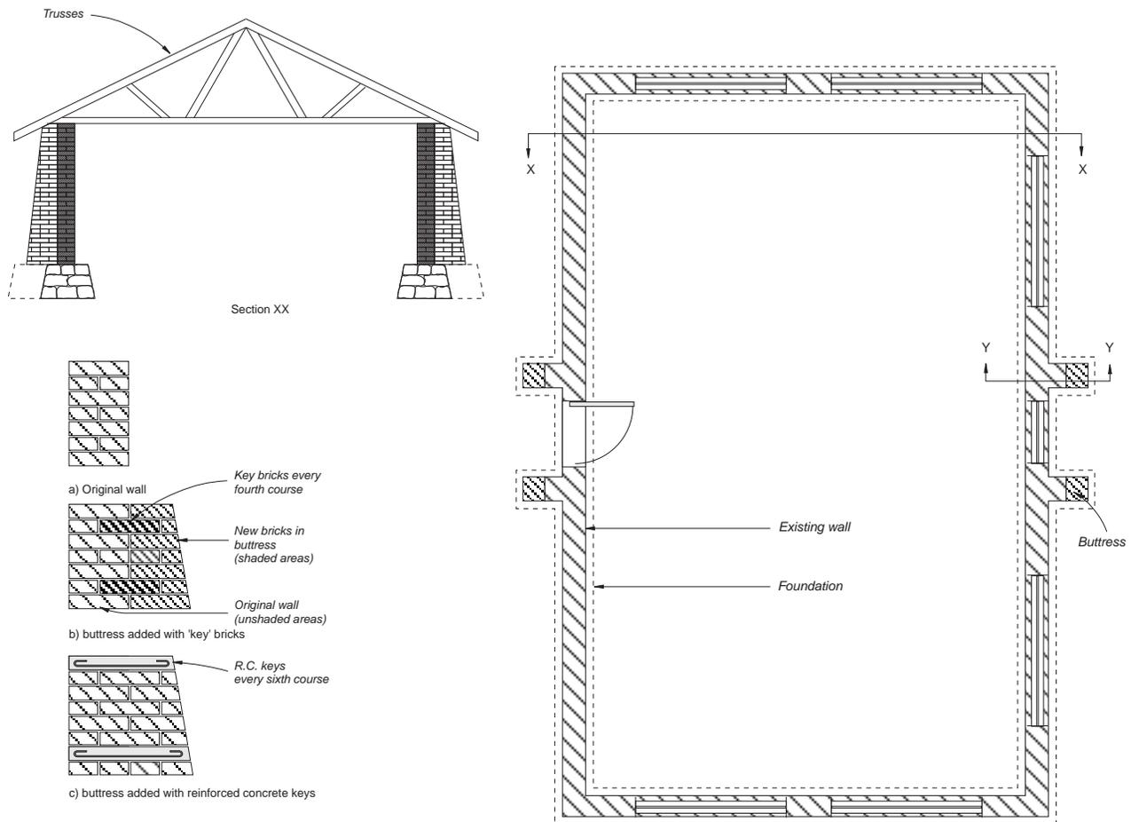
Fig. 79 : Strengthening existing wall with buttressing
