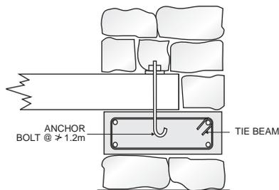
Fig. 62 : Anchorage of timber joists into RC band using anchor bars
