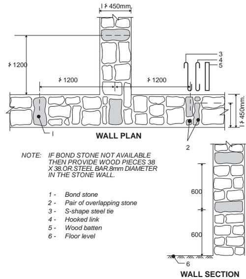
Fig. 45 : Random rubble masonry with "through" stone or other bonding elements
