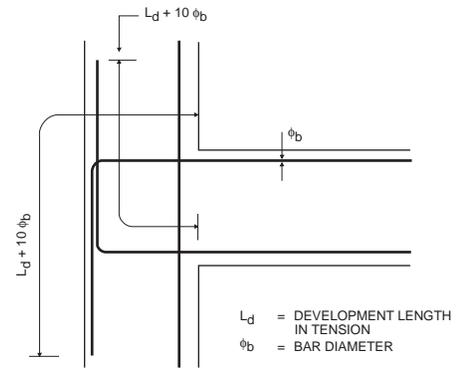
Fig. 52 : Anchorage beam bars in an external joint
