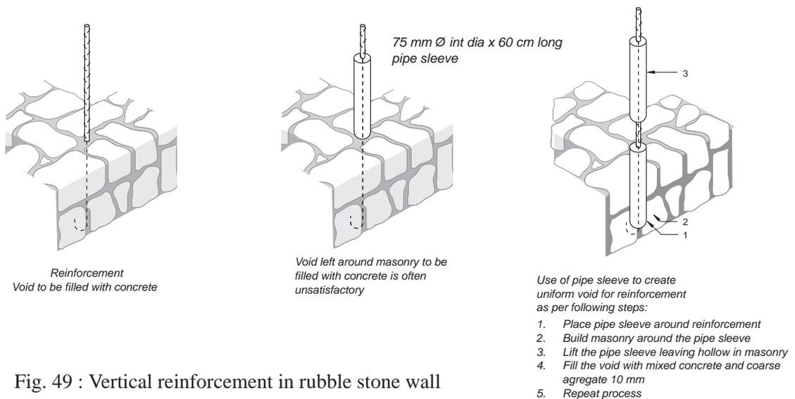
**Fig. 49 : Vertical reinforcement in rubble stone wall**
