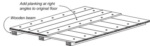
Fig. 73 : Stiffening of wooden floor by wooden planks
