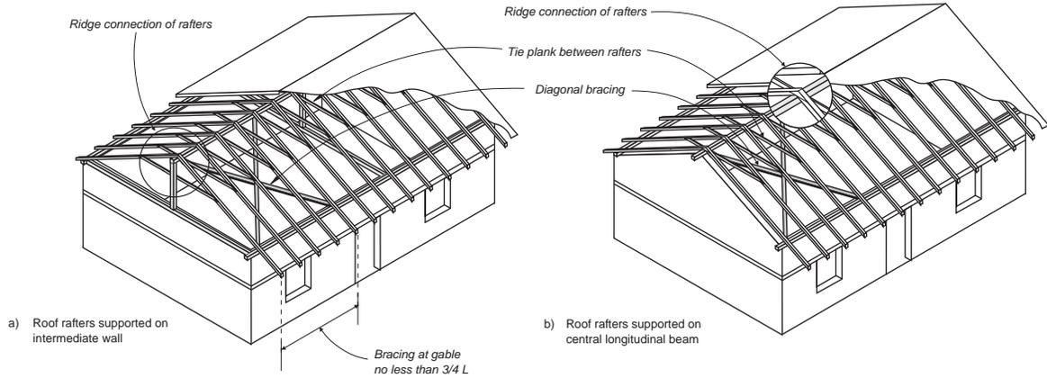
Fig. 67 : Use of A-type trusses to reduce thrust on wall
