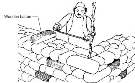
Fig. 46 : Wall junction strengthening
