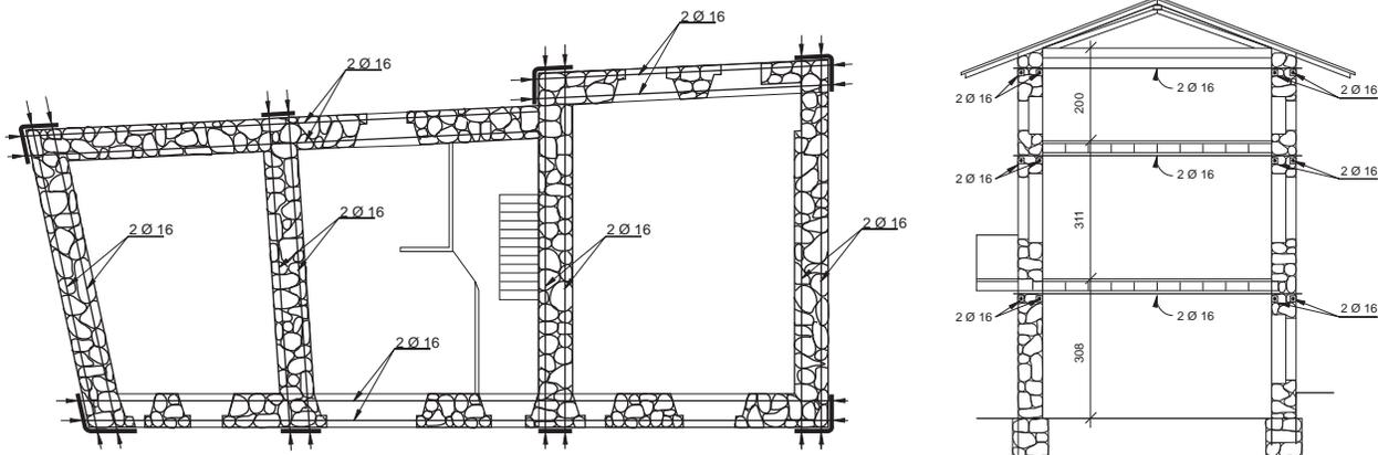
Fig. 82 : Strengthening walls by prestressing
