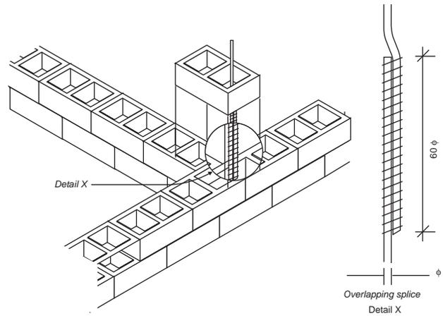
Fig. 38 : Vertical bar in hollow concrete and stonecrete block
