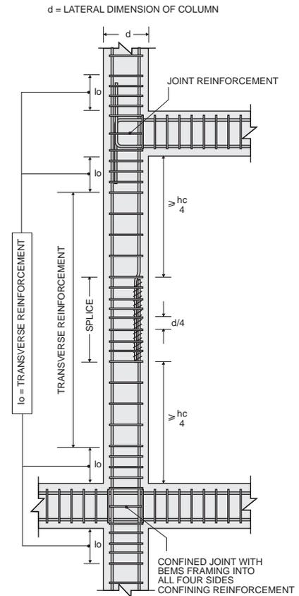
Fig. 58 : Column and joint detailing
