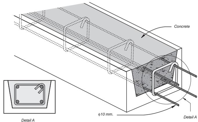
Fig. 37 : Section of Horizontal band
