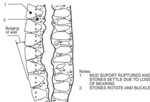
Fig. 44 : Stone wall delamination with buckled wythes
