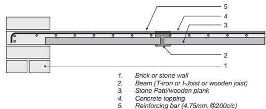
Fig. 65 : Floor stiffening using RC topping
