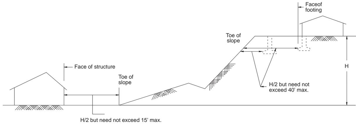
Fig. 17 : Preparing a building site in a sloping terrain
