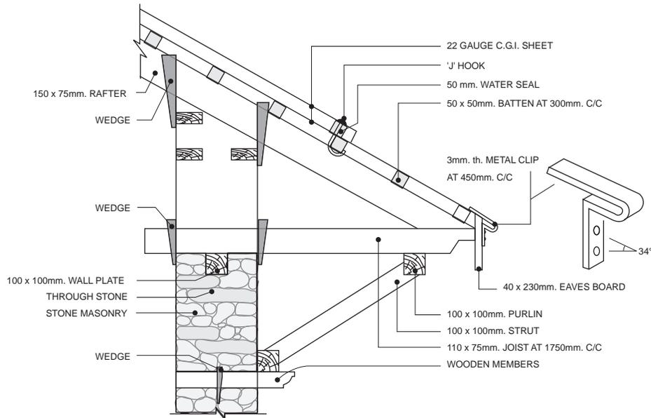
Fig. 69 : Anchorage of timber joists with wall using wedges
