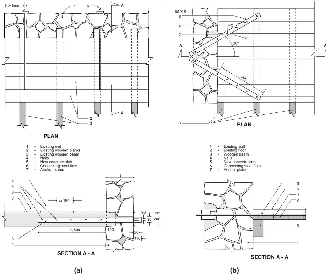
Fig. 76 : Connection of floor with wall (a-b)
