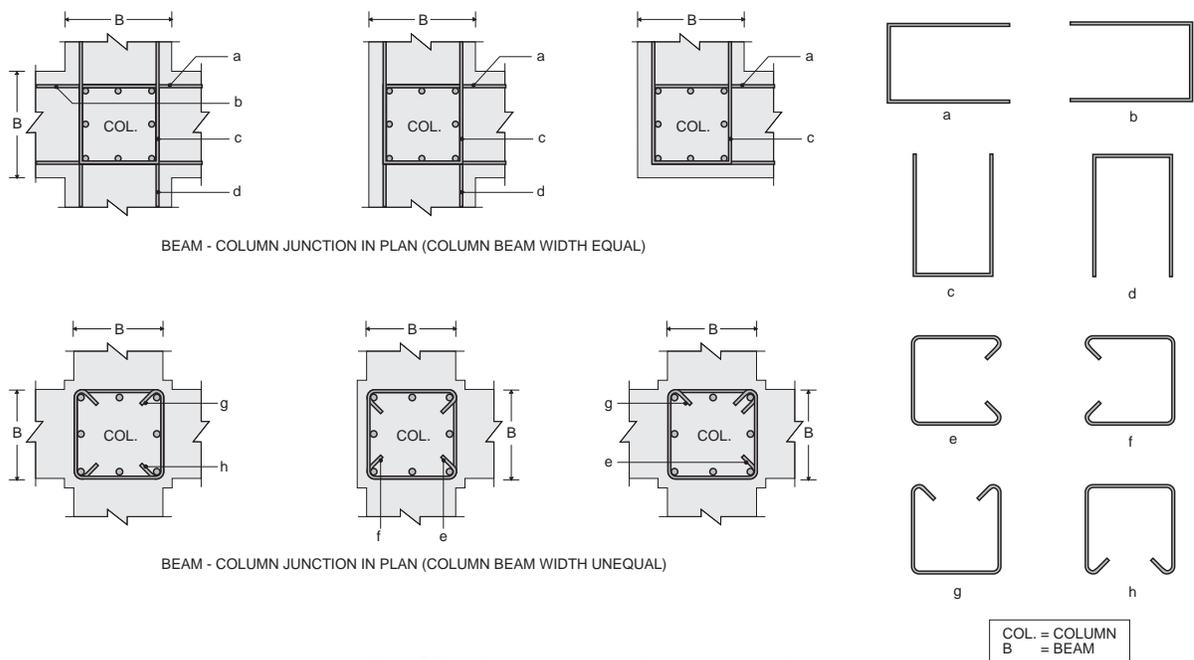
Fig. 59 : Hoop stirrups for joints in frame
