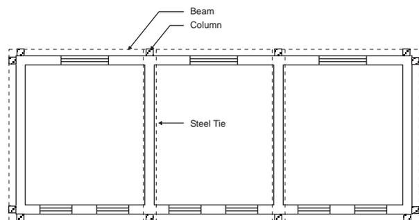
Fig. 85 : Column and beam strengthening technique
