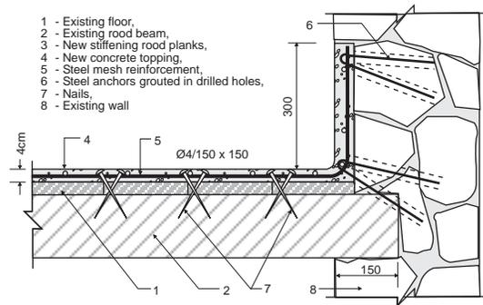
Fig. 75 : Stiffening the existing floor/flat roof by bracing
