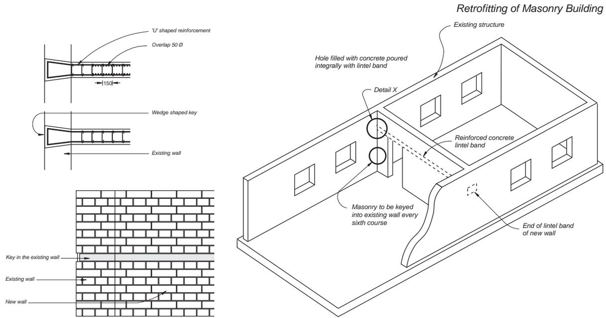
Fig. 78 : Inserting internal cross wall
