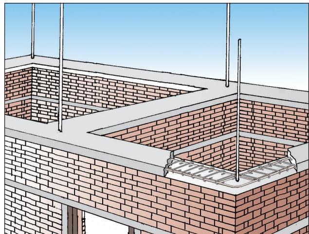
Fig. 35 : Reinforced concrete band
