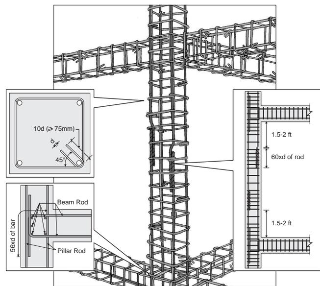
Fig. 56 : Lap splice in beam
