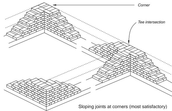
Fig. 30 : Staggered toothed wall joint
