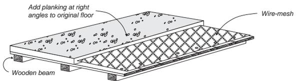
Fig. 74 : Stiffening of wooden floor by RC topping
