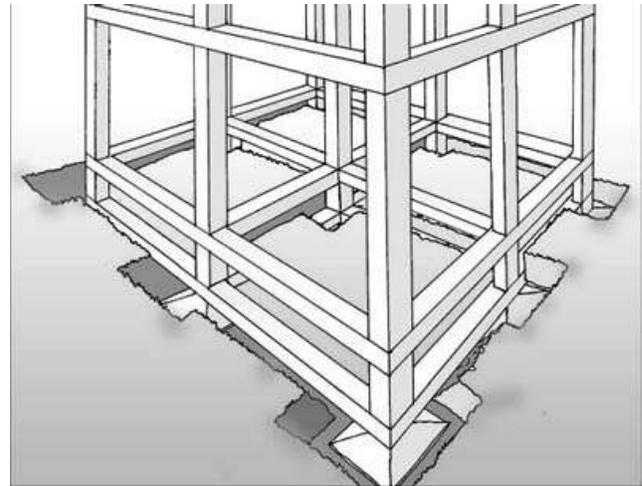
Fig. 50 : Tying up isolating footings
