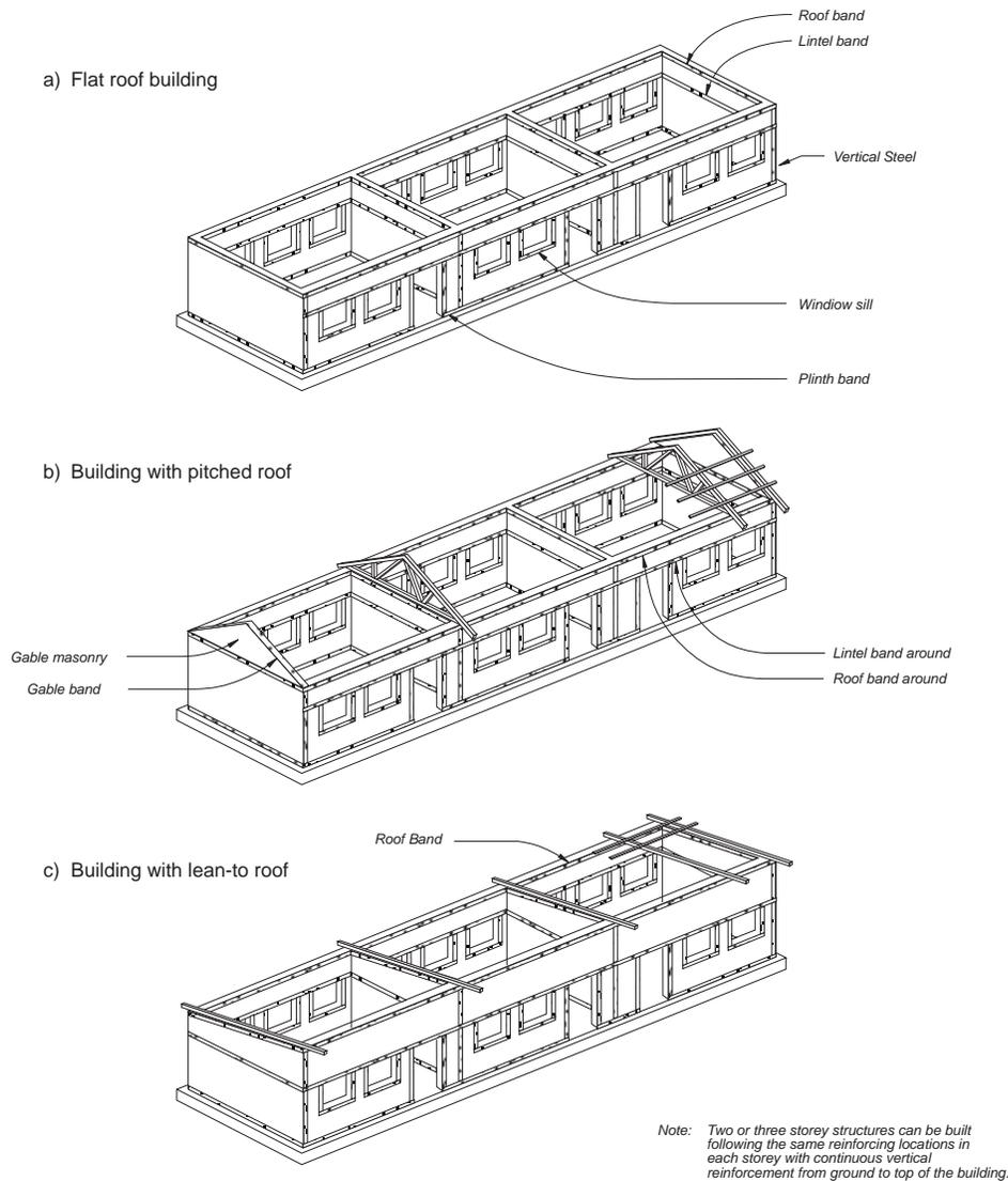
Fig. 23 : Locations for reinforcing
