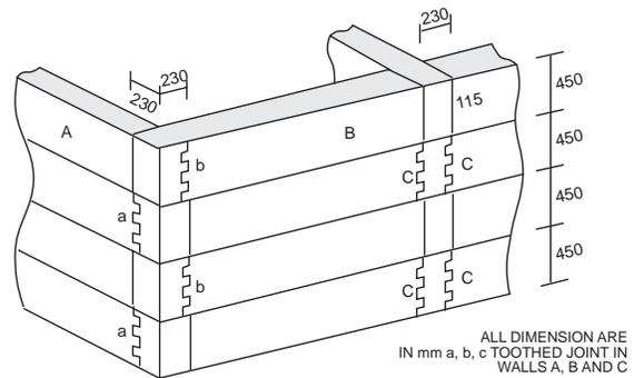
Fig. 31 : Stepped wall joint stitching
