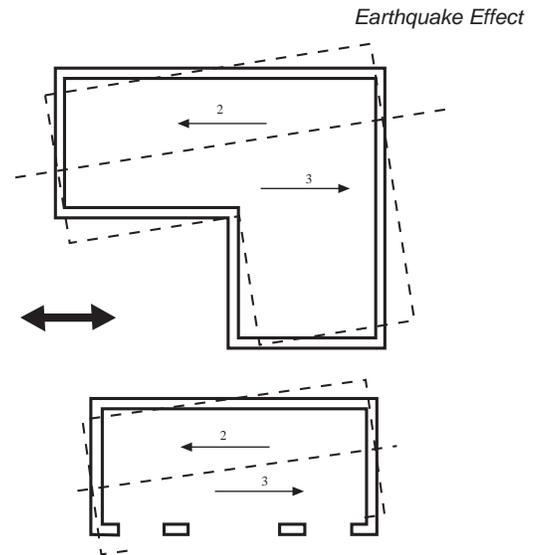
Fig. 14: Torsion in Unsymmetrical Plan building
