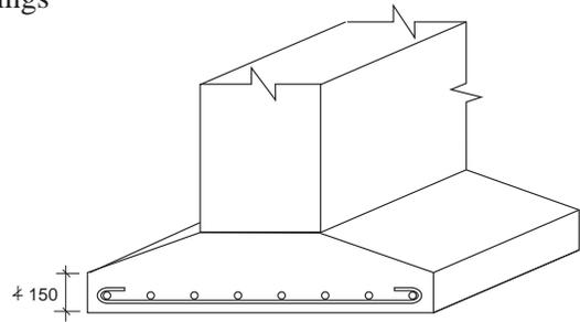
Fig. 25 : Construction of strip foundation in RC
