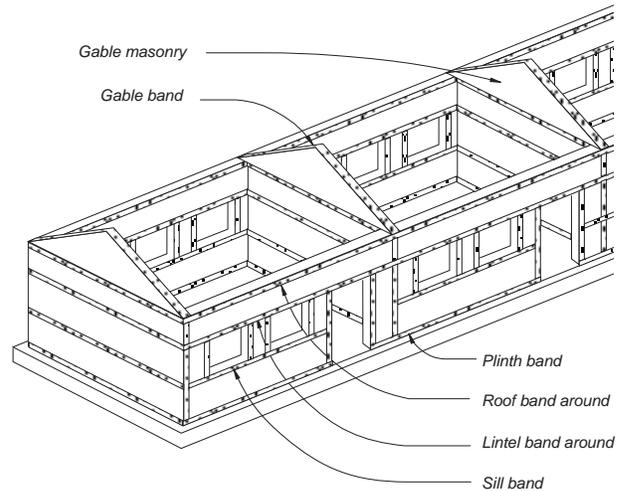
Fig. 34 : Bands at different levels
