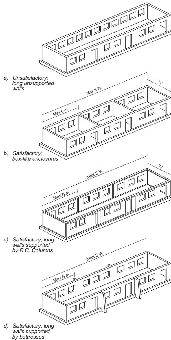
Fig. 22 : Lateral supports to long walls
