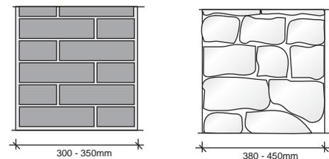
Fig. 40 : Cross section of stone wall
