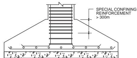
Fig. 51 : Provision of special confining reinforcement into footing
