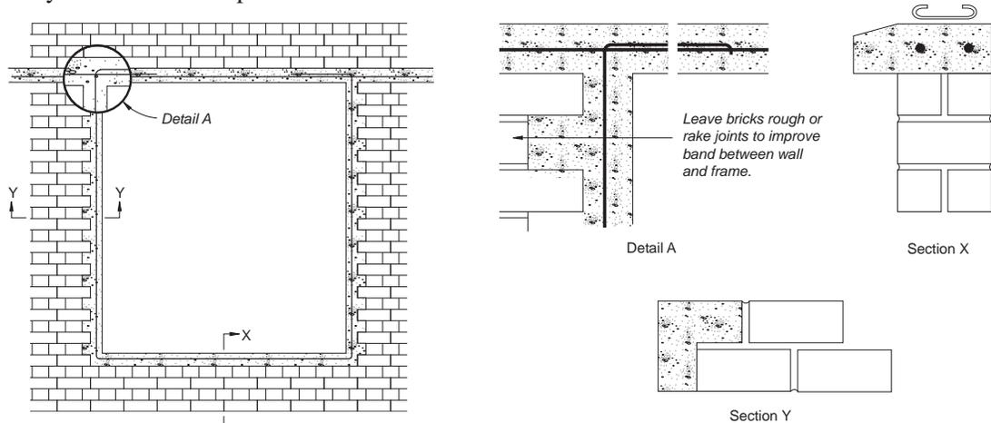
Fig. 29 : Reinforcing of openings
