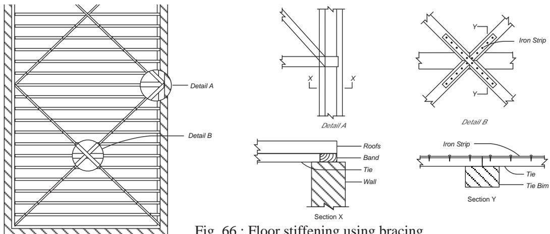
Fig. 66 : Floor stiffening using bracing
