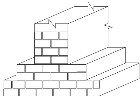
Fig. 27 : Masonry strip footing
