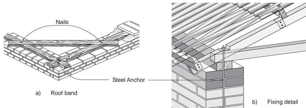
Fig. 68 : Anchorage of timber rafters into RC band using anchor bars
