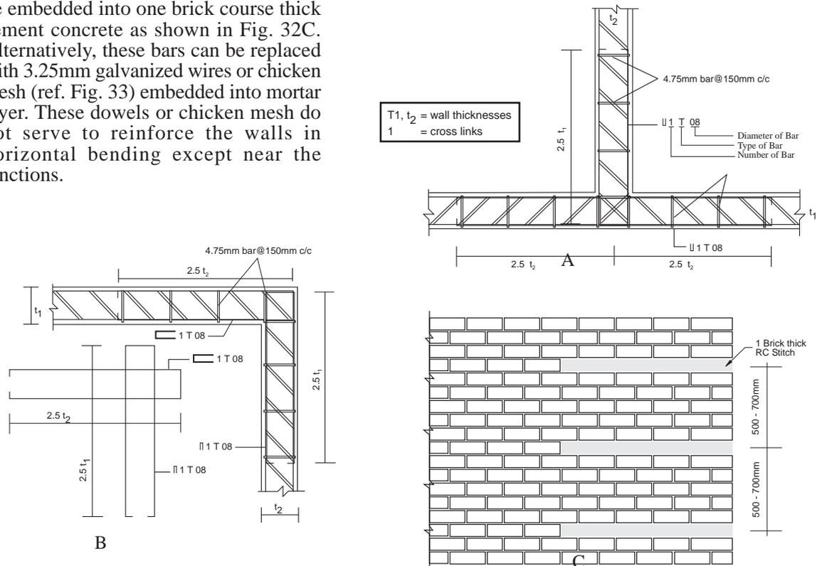
Fig. 32 : Joint strengthening by dowel reinforcement placed in one joint
