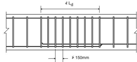
Fig. 53 : Lap splice in beam
