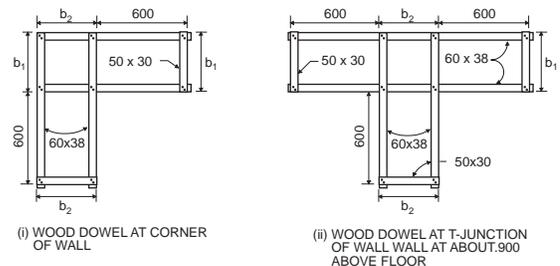
Fig. 47 : Detail of timber stitches
