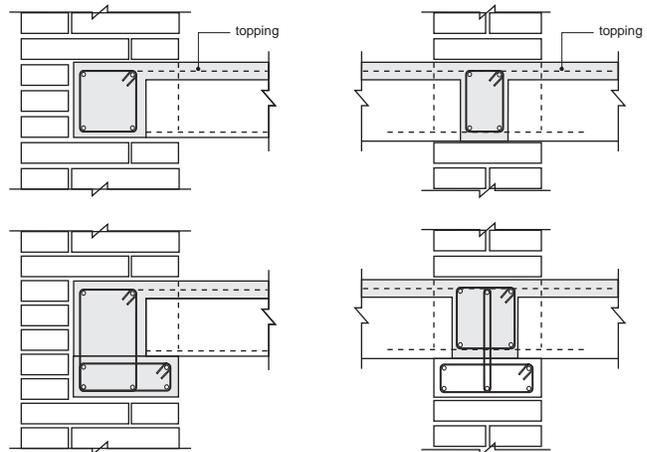
Fig. 60 : Precast slab with reinforced concrete topping
