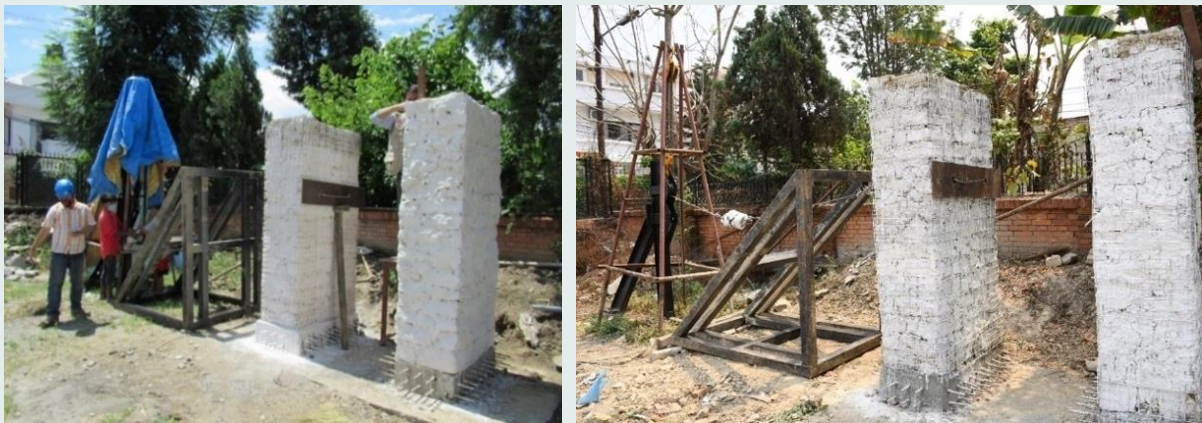
Pull down test of Retrofitted Stone-in-Mud Masonry Walls
