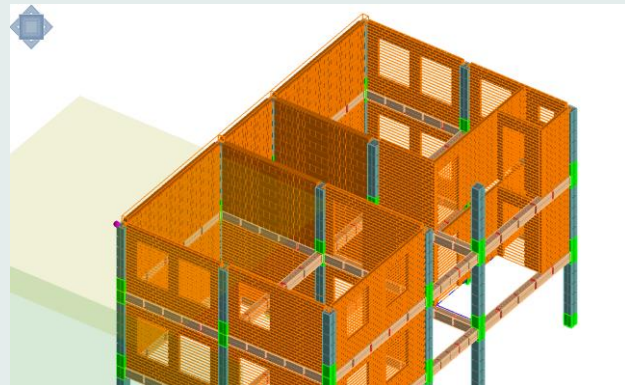
Ongoing modelling works for fragility assessment of RC structures (2)
